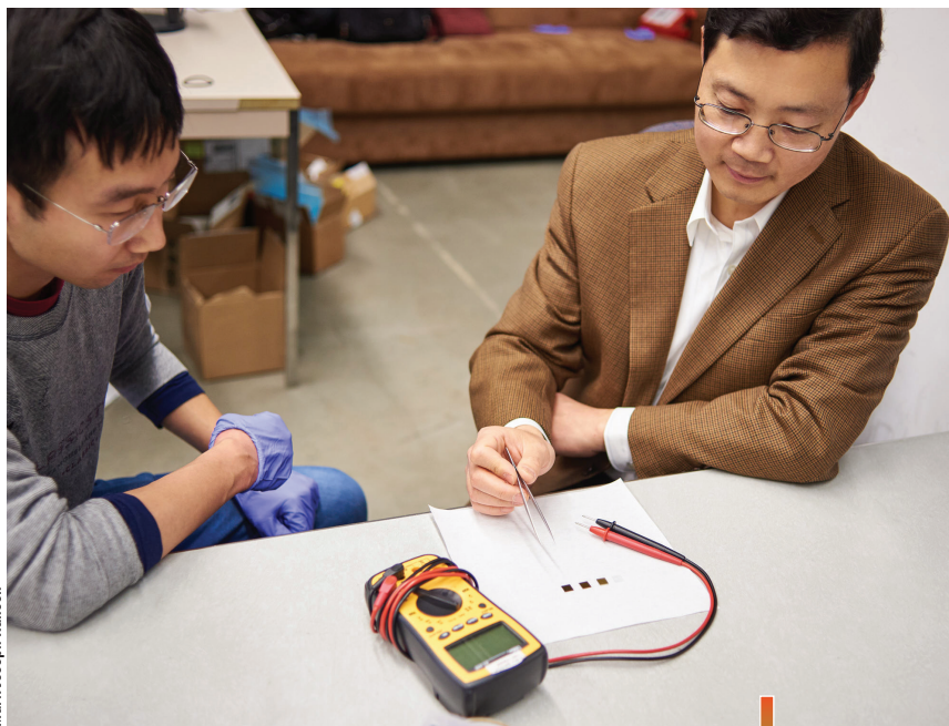
Kechao Tang and Junqiao Wu examine samples of ultra-thin vanadium dioxide films that switch automatically between conducting heat and insulating against it.
