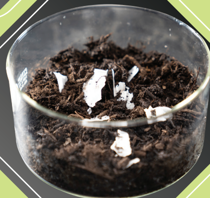
Top to bottom: Graduate student Ivan Jayapurna prepares a sample film of polylactic acid plastic; an undegraded film of polylactic acid plastic; biodegraded fragments of polylactic acid plastic.
