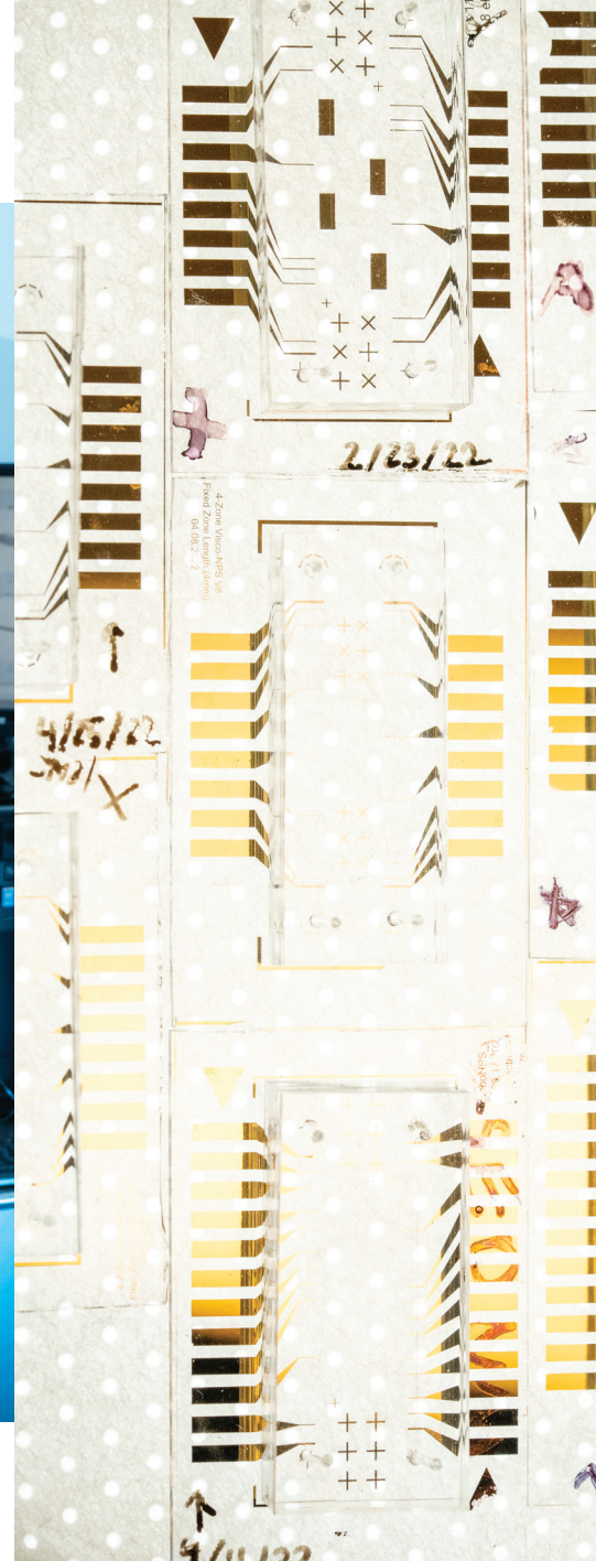
Mechanical engineering professor Lydia Sohn holds a petri dish containing mechano-node pore sensing (NPS) devices, which are shown in a close-up image, right.
